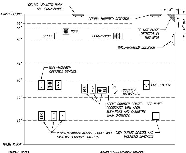
I. MOUNTING HEIGHTS SHOWN IN THIS DETAIL ARE TYPICAL UNLESS OTHERWISE NOTED ON THE PLANS 2. SEE ARCHITECTURAL ELEVATIONS FOR SPECIAL
